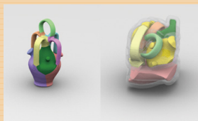
図1 Level-Set-Based Partitioning and Packing Optimization of a Printable Model
